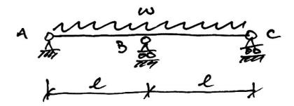
8. (Summer 2008) For the prismatic beam of Fig. Q3(b), using Macaulay's Method, find the vertical deflection at *C* in terms of *EI*.
