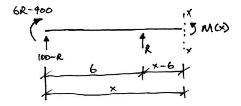
Proceeding as usual, we take moments about the cut, being careful to properly locate the moment reaction at *A* using the correct discontinuity function format:
