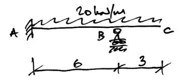
6. For the beam shown, find the reactions and draw the bending moment, shear force, and deflected shape diagrams. Determine the maximum deflection and the rotations at *A*, *B*, and *C* in terms of *EI*.
