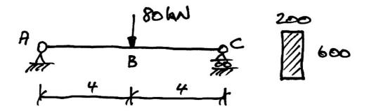
For this and subsequent problems, we need to know how to determine the flexural rigidity, *EI*, whilst being aware of the unit conversions required:
