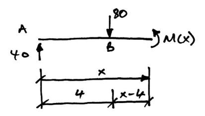
Note that in this diagram we have taken the cut so that all loading is accounted for. Taking moments about the cut, we have:
