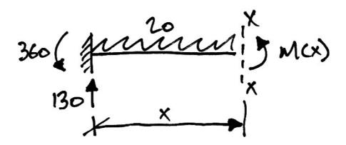
Note that even though it is apparent that there will be tension on the top of the cantilever, we have retained our sign convention by taking M(x) as tension on the bottom. Taking moments about the cut:
