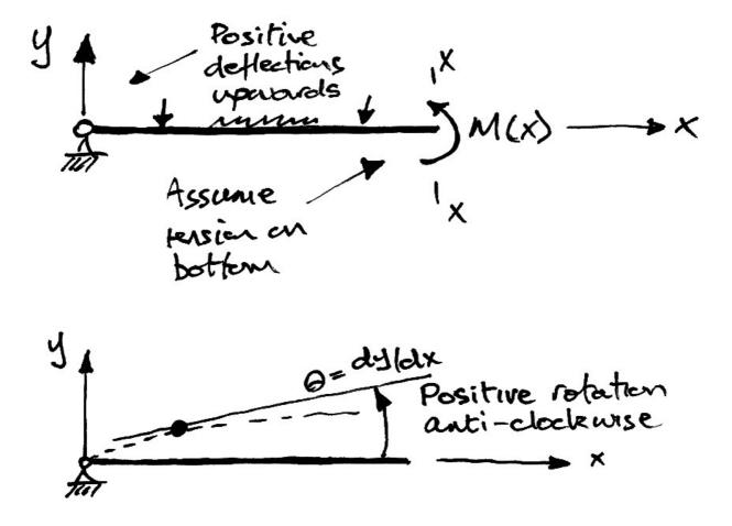
When it comes to frame members at an angle, we just imagine the above diagrams rotated to the angle of the member.
