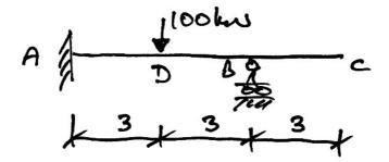
4. For the beam shown, find the reactions and draw the bending moment, shear force, and deflected shape diagrams. Determine the maximum deflection and rotation at *B* in terms of *EI*.
