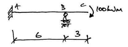
5. For the beam shown, find the reactions and draw the bending moment, shear force, and deflected shape diagrams. Determine the maximum deflection and rotation at *B* in terms of *EI*.
