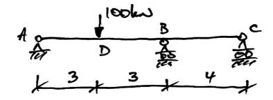
7. For the beam shown, find the reactions and draw the bending moment, shear force, and deflected shape diagrams. Determine the maximum deflection and the rotations at *A*, *B*, and *C* in terms of *EI*.
